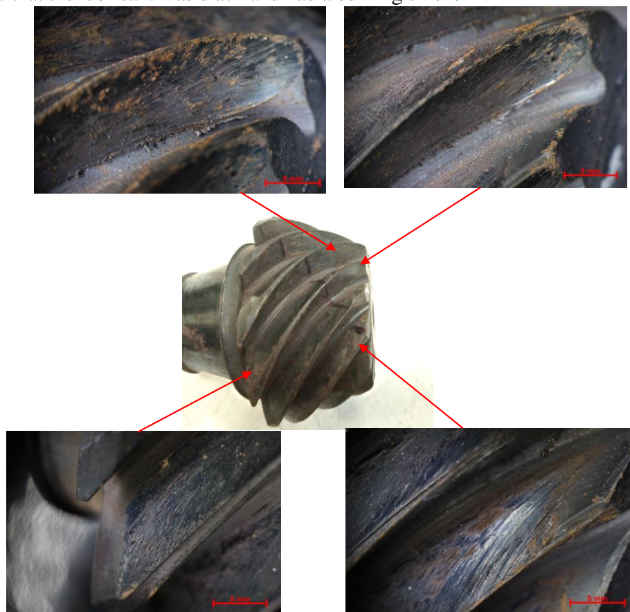
Figure 4 The burnt appearance of damaged pinion gear
