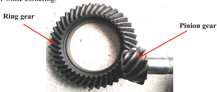
Figure 1 Rear differential model of hypoid bevel gear
