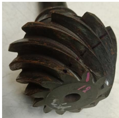
Figure 2 The wear and burn marks of rear differential contact
